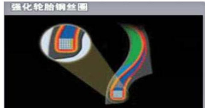
3. The latest tire contour design simulated by the computer greatly reduces the energy generated by the strain of the belt and fetal.
