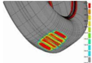
4. The most optimizing design of tire shoulder can avoid the concentration caused by the abnormal pressure of the punctured tire.
