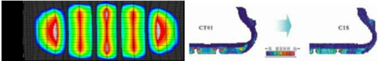
2. Using CASPAN system to measure the contact shape and pressure ensures that when the tire contacts the ground, the rigidity of the rubber remains consistent and vibration amplitude tends to balance, so as to reduce the noise which is caused by the pattern.
