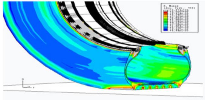
2. Special methods of improving the non-contact part of the shoulder greatly decrease the accumulation of excessive heat in this part. With the dropping of tread temperature, the fatigue of tread rubber has been reduced greatly, which ensures durability and high-spe.
